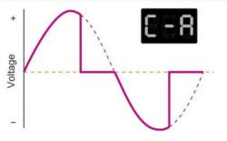
Lamps with electronic transformers Extremely silent operation Smoother dimming down to 5% In general better results with LED lamps
