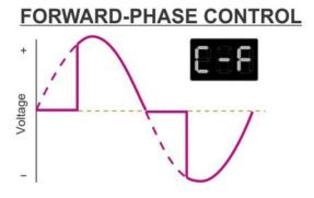
For Incandescent lamps (better energy efficiency) Lamps with magnetic transformers Some LED lamps / drivers
